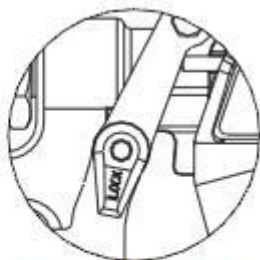
Trigger unlocked (gun will spray)
